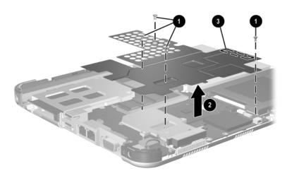
Removing the System Board Shield
